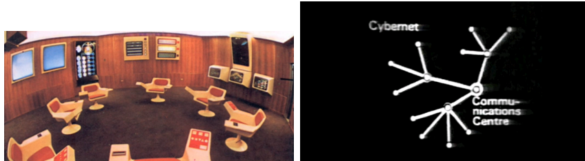
Figure 1.1: Left is the control room of the Chilean cybersyn system. To the right is a representation of the cybernet computer network used by the system to contact its sensors and regulators.
